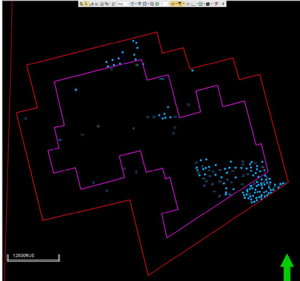
Figure 31—Map view of the 164 petrophysically QCd, neutron-density calibrated porosity log curve control points for porosity modeling.
