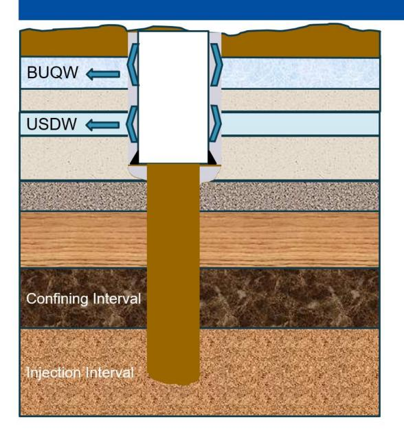
§5.203 (f)(1)(D) Before **long string** casing is installed, the operator must run logs appropriate to the geology, such as resistivity, spontaneous potential, porosity, caliper, gamma ray, and fracture finder logs, to gather data necessary to verify the characterization of the geology and hydrology.
