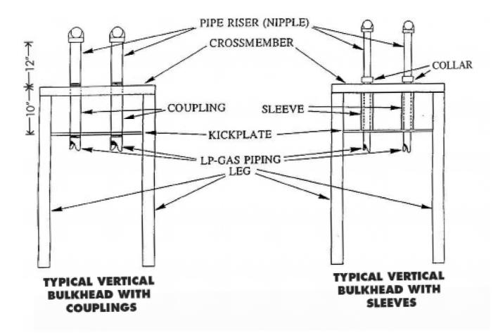
(A) Six-inch steel channel iron shall be used.
