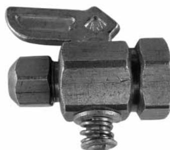
**Figure 2** Unapproved shutoff valve. The spring and nut are located outside the valve body.
