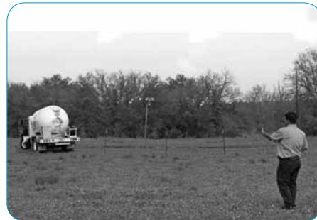
Testing Off-Truck Remote Emergency Shutdown Device
