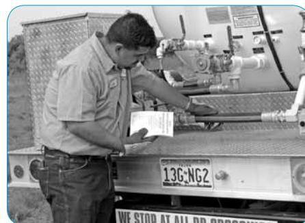
Inspecting Hose Reels, Meter and Connecting Piping
